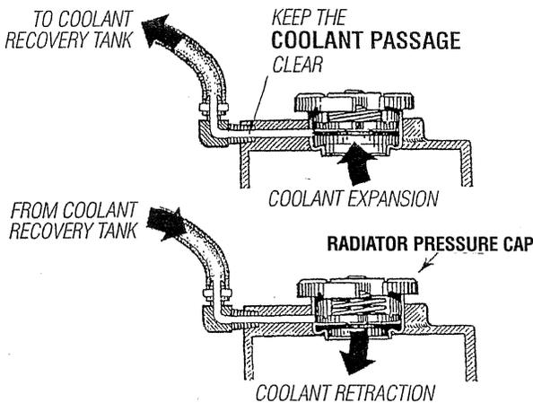
**NOTE:** Periodically check the condition of the radiator coolant pressure cap. Ensure the upper and lower rubber seals are in good condition. Check to ensure the vacuum valve opens and closes tightly. Carry a spare cap. Check also to ensure the coolant passage is clear so coolant within the system is able to expand and contract to and from the coolant recovery tank.
