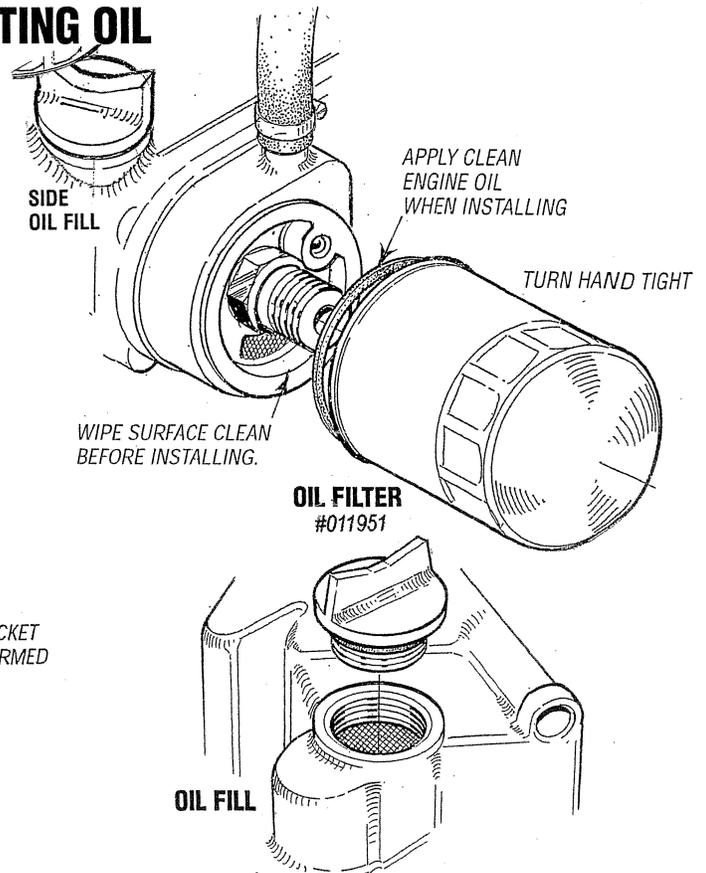
**NOTE:** Generic filters are not recommended, as the material standards or diameters of important items on generic parts might be entirely different from genuine parts. Immediately after an oil filter change and oil fill, run the engine to make sure the oil pressure is normal and that there are no oil leaks around the new oil filter.
