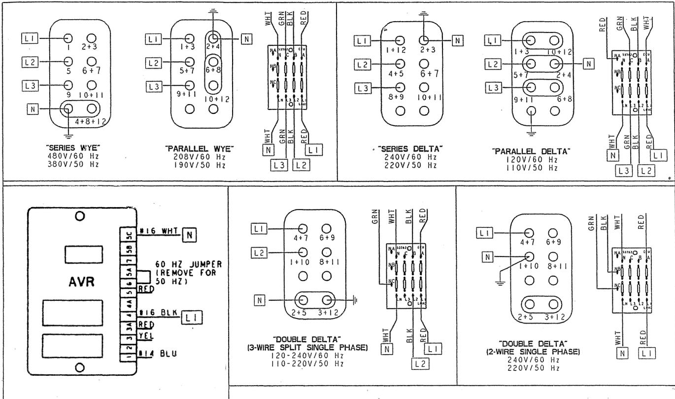
**NOTE:** Tie off the L3 sensing connection when not used.
