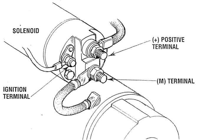
To test the ignition circuit, locate the ignition(s) terminal (it is one of the small terminal studs and is wired to the ignition circuit). Use a screwdriver, don't touch the blade, to jump from that ignition terminal to the positive battery connection terminal on the solenoid.
