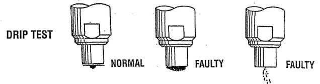
2. Apply the pressure of 1635 kg/cm<sup>2</sup> (115 lb/in<sup>2</sup>) to nozzle by operating the hand lever, and check the drips from the nozzle tip. If it drips or has a large accumulation of fuel on the bottom, it is considered defective and should be replaced. A very small amount of fuel may sometimes remain on the tip of the nozzle; however, this does not indicate a defect.
