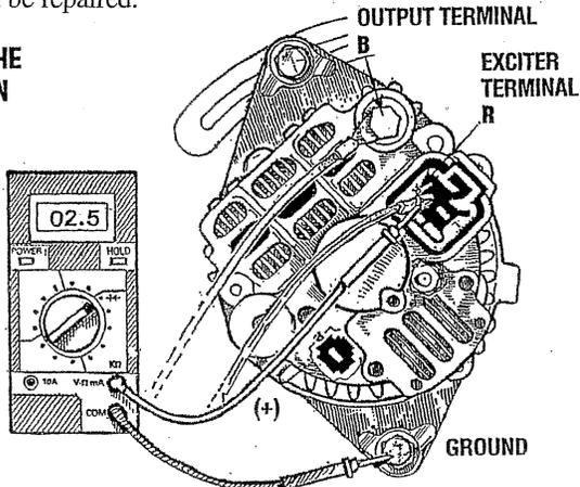
3. If no reading is obtained, an open exists in the alternator/excitation lead. Disconnect the lead from the excitation terminal **R**. Trace the lead to determine the fault and correct.
