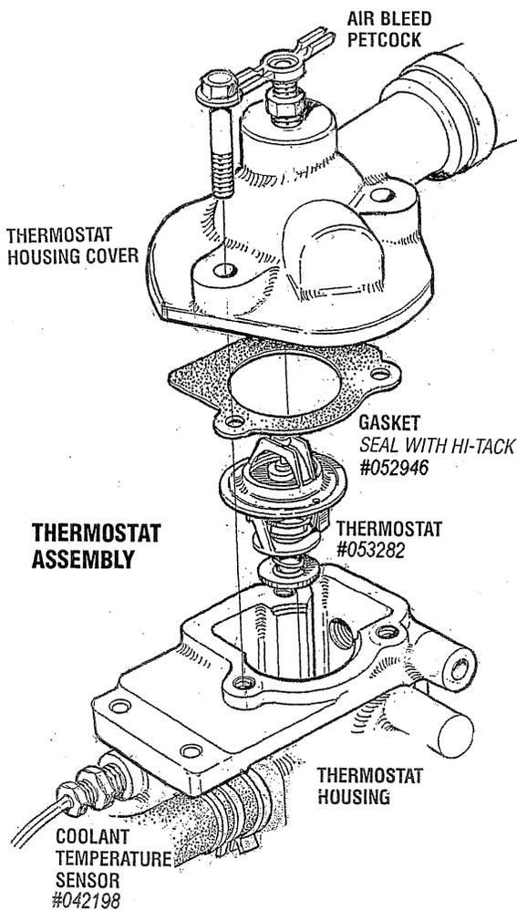
2. **Remove the thermostat housing cover.** Remove the hose clamp and twist the hose off the connection of the housing. Remove the three bolts holding the housing to the thermostat base. Lift the housing off the base. This will give you access to the housing gasket and thermostat.
