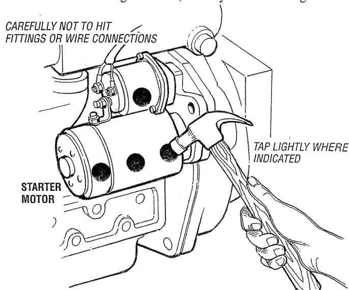
If that fails, turn the battery switch on and have a crew member turn the ignition on and off rapidly as you tap again with the hammer. This may loosen the brushes and allow contact to start the engine. When you reach a repair facility, the starter will need to be repaired.
