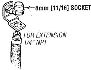
REMOVE USING AN 8MM (11/16") SOCKET TO DRAIN THE OIL OR PUMP THE WARMED OIL UP THRU THE HOSE.
