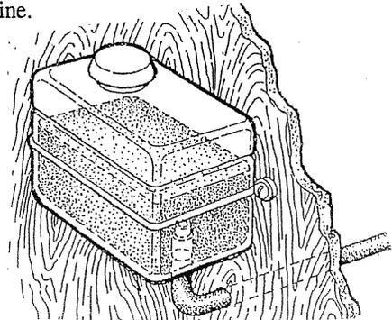
**NOTE:** *This tank, with its short run of plastic hose, is best located at or above the level of the engine's manifold, but it can be located below the level of the engine's manifold if the particular installation makes this necessary.*
