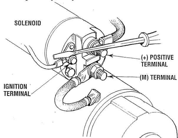
If nothing happens at all, the solenoid is not getting current.. Check the battery isolation switch and inspect the wiring connections. It is also possible that the solenoid is defective.
